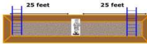
Egress - Trench Excavation 1926.651(c)(2)
