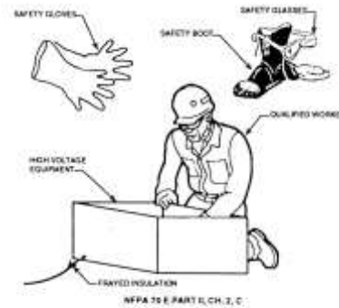
Figure 8-3. All employees are required to wear protective equipment to protect their eyes from flashes, arcs, etc.
